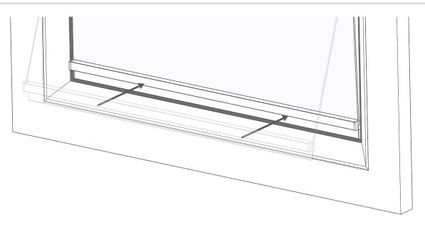
Pull the bottom rail out towards the bottom of the window, stretching out the cords. Just like the top rail, line up the bottom rail carefully with the edge of the visible glass and press it into place.
