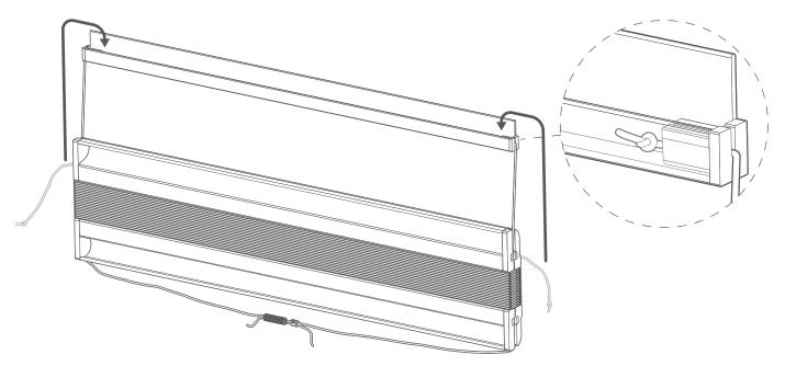
Take the two knotted ends of the top cords at either side of the blind, and hook each knot over and into the slots at the ends of the top rail, so the blind is suspended from the top rail by those two cords. Hold it steady as you continue, so the cords don't slip out.
