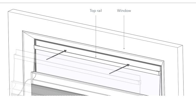
Carefully line up the top rail with the top of the visible glass. Make sure that the top of the top rail is flush with the edge of the rubber seal, if the seal is visible, or the edge of the frame if it is not. Press the adhesive-backed v to the glass and hold until it feels secure.
