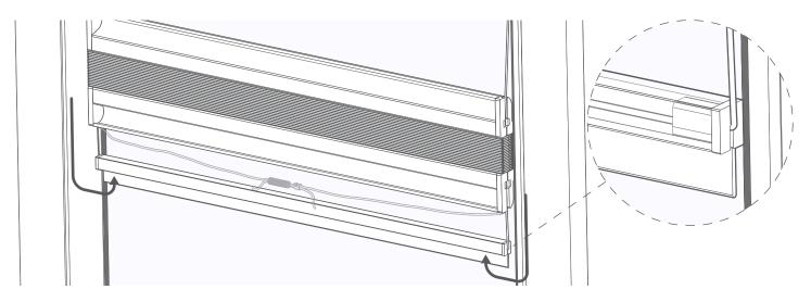
Take the bottom cord and loop it under the bottom rail, so that the cord rests in the notches at the ends of the rail. Try to keep the spring to which the ends of the cords are attached in roughly the centre. The cords and spring should tuck neatly behind the rail.
