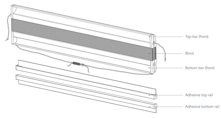
When you first unwrap the blind you'll find that it's in 3 parts - the blind itself, and the top and bottom adhesive rails from which the blind will be suspended.
